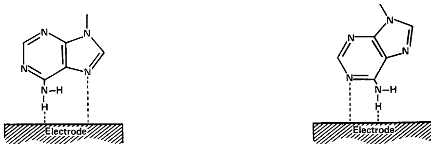
Figure 11. Possible modes of binding of adenine to the mercury electrode surface when in perpendicular orientation in region of anomalous capacitance pits
